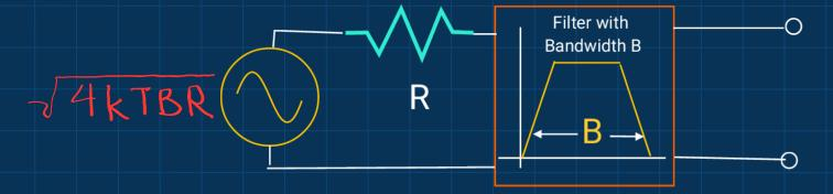
The available noise power density from a resistor is.
