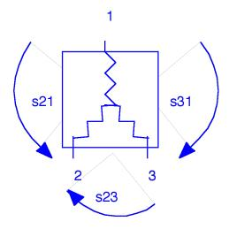
Make a vector measurement, i.e. magnitude and phase, of s21 and s31. Adjust the electrical delay for channel 2 under the scale menu until the phase is flat. Use the same electrical delay for both measurements. Sketch the amplitude and phase of each measurement. What is the amplitude and phase balance? What is the electrical delay of the device?
