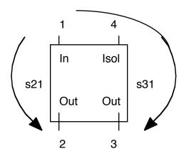
The 180-degree Hybrid is a four port device. Make a vector measurement, i.e. magnitude and phase, of s21 and s31. Adjust the electrical delay as before for the phase signal until the phase is flat. Use the same delay value for both s21 and s31. Sketch the amplitude and phase of each measurement. What is the amplitude and phase balance?
