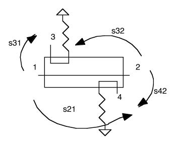
Measure the magnitude transfer function parameters s31 and s42. This is called the coupling factor. Sketch the results and state the average coupling factor for the device. What is the coupling bandwidth of the device, i.e. 3 dB below the coupling value?
