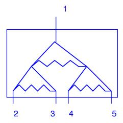
Repeat the Wilkinson splitter experiment with the 4 way Wilkinson splitter. Pay special attention to the isolation measurements between s21, s31 and s41, s51.
