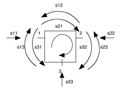
The circulator is a three port device. Measure the magnitude function of all nine s parameters as shown in the diagram. Use channel 1 for s11, s22, s33 and channel 2 for the other six parameters, s21, s12, s23, s32, s13, s31. Sketch the results and list rough magnitude values in the form of a 3X3 s matrix. From inspection of the parameters, describe the signal flow through the device.
