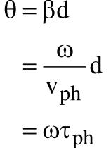
The <u>phase</u> delay of a device is defined as:
