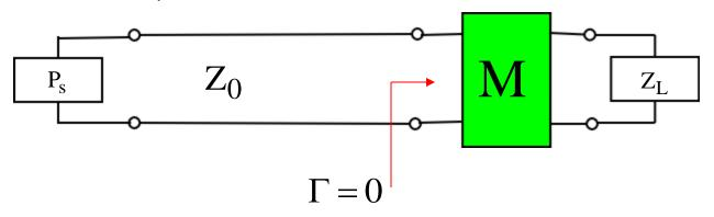
Typically we only want to use lossless devices such as capacitors, inductors, transmission lines, in our matching network so that we do not dissipate any power in the network and deliver all the available power to the load.
