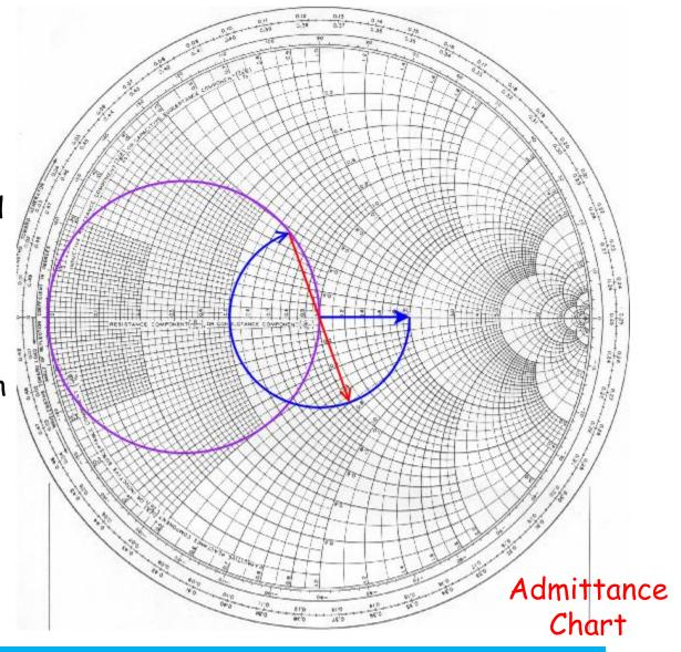
An open stub of zero length has an admittance=j0.0
