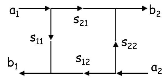
$s_{11}$  and  $s_{22}$  can be thought of as reflection coefficients
