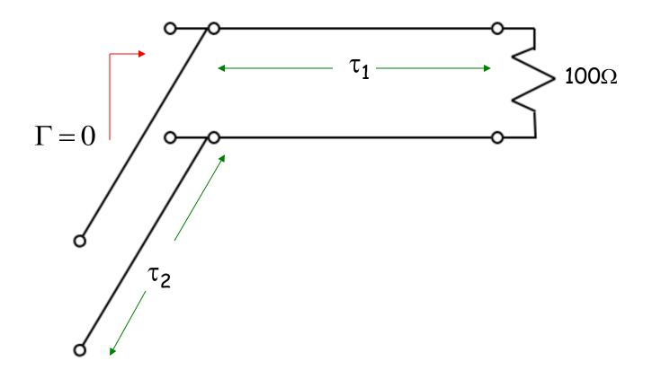
Match  $100\Omega$  load to a  $50\Omega$  system at 100MHz using two transmission lines connected in parallel
