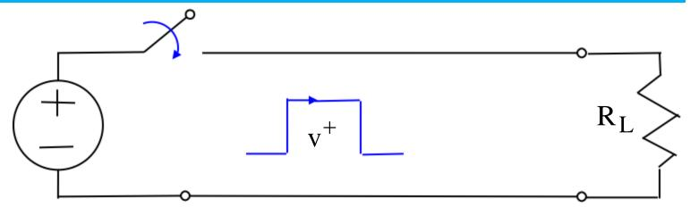
Pulse travels down the transmission line as a forward going wave only ( $v^+$ ). However, when the pulse reaches the load resistor:
