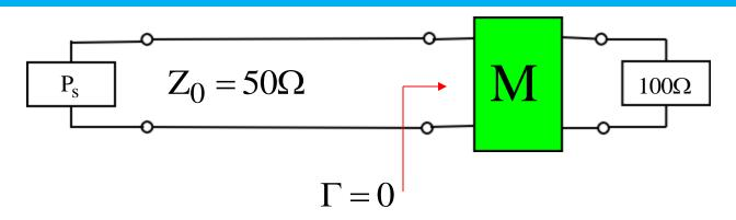
Match 100  $\Omega$  load to a 50  $\Omega$  system at 100 MHz
